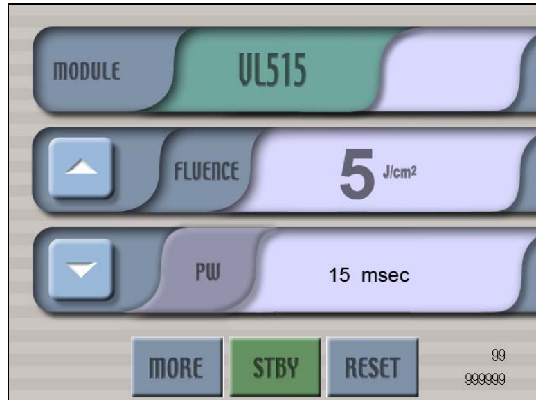
Figure 4-2: SVL Module Operating Screen
