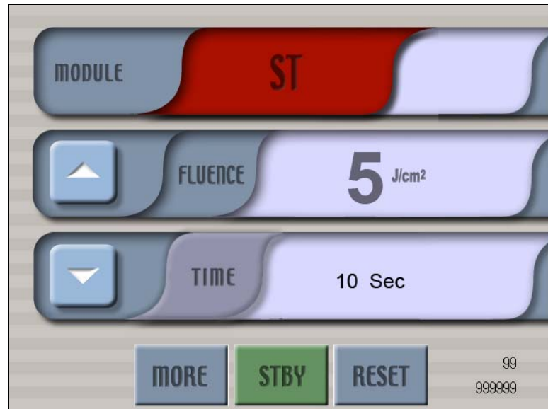
Figure 8-2: ST Module Operating Screen
