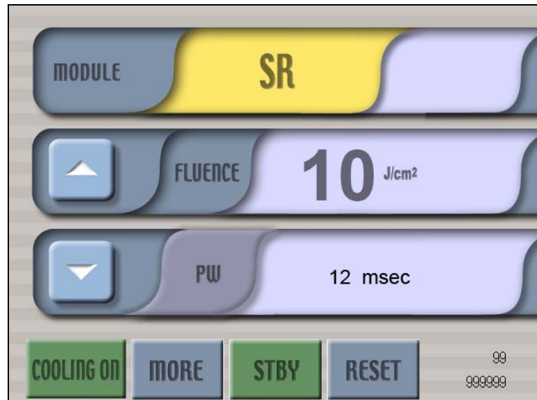
Figure 12-2: SR Cooled Module Operating Screen
