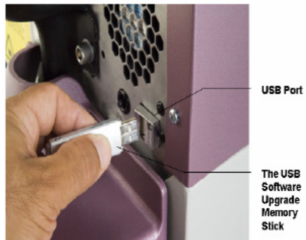
Figure 6.1: Laser System Software Upgrade USB Port and Memory Stick
