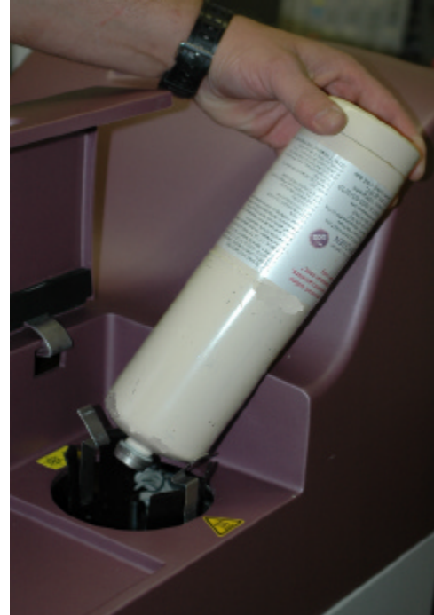
Figure 6.11: Cryogen Canister Replacement
