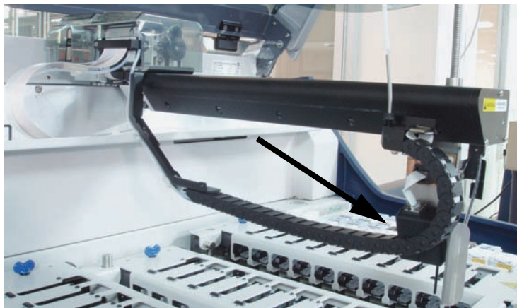
Figure 3: Photo of the robot with the ID imager indicated by the arrow
