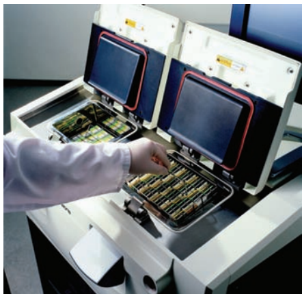
Figure 11: Placing a basket into a retort
