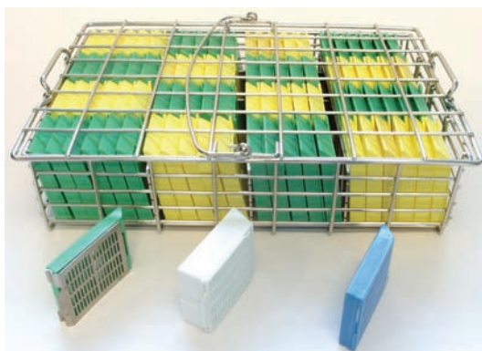
Figure 8: Peloris high capacity basket with some of the compatible cassette types
