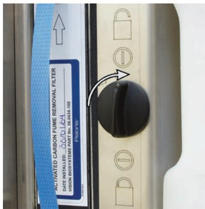
Figure 22: Unlocking the filter
