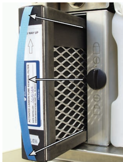
Figure 23: Removing the filter
