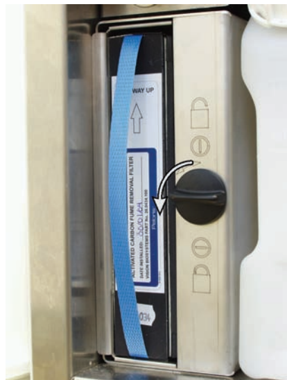
Figure 25: Locking the filter
