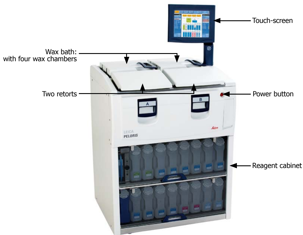
Figure 1. PELORIS tissue processor – main features
