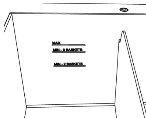
Figure 4. Wax chamber fill levels
