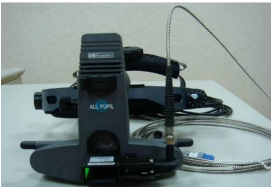
Figure 5.19 LIO LDU fiber connection
