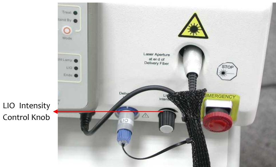
Figure 5.31 (a) Fiber and Delivery Key fitted to Console Front Panel
