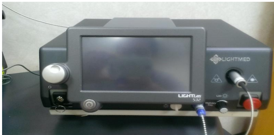
Figure 5.21 (c) Sample of Delivery Fiber and Delivery Key Connection
