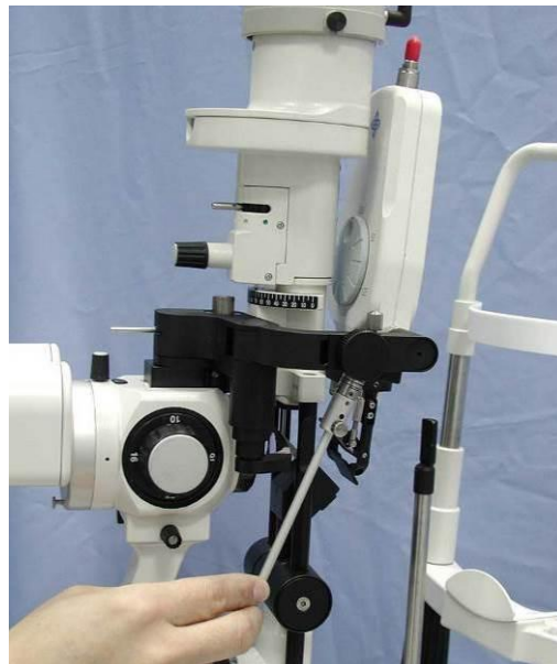
Figure 5.29 Old type version Adjusting Micromanipulator Arm to verify Laser Spot is in the Aperture Center
