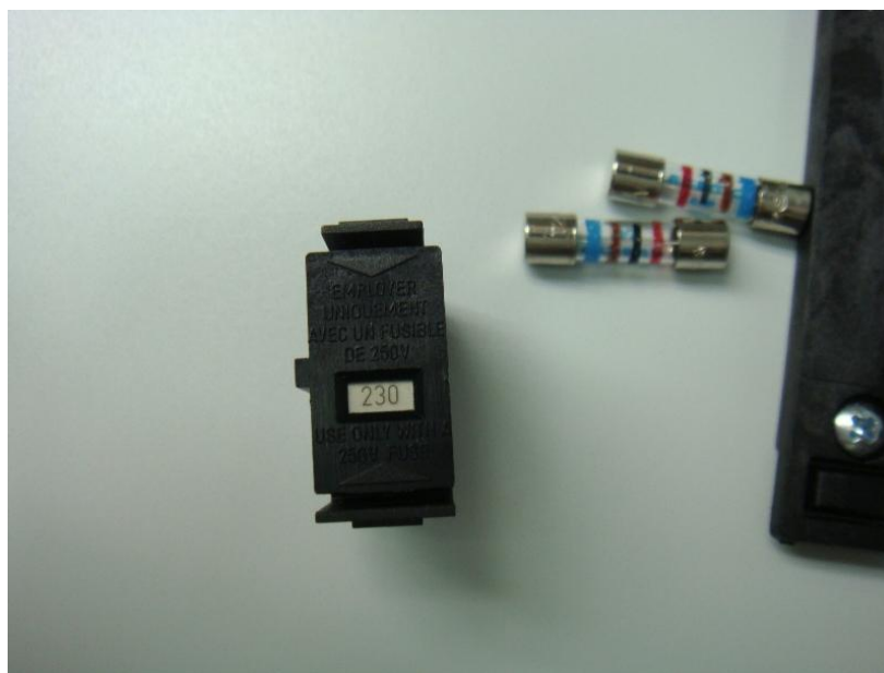
Figure 5.5 (c) Removal of fuses and check the fuses rate
