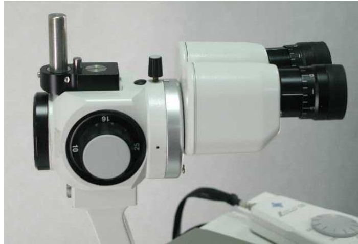
Figure 5.15 (a) Haag Streit Attaching Tonometer mount ready for Attachment LDU
