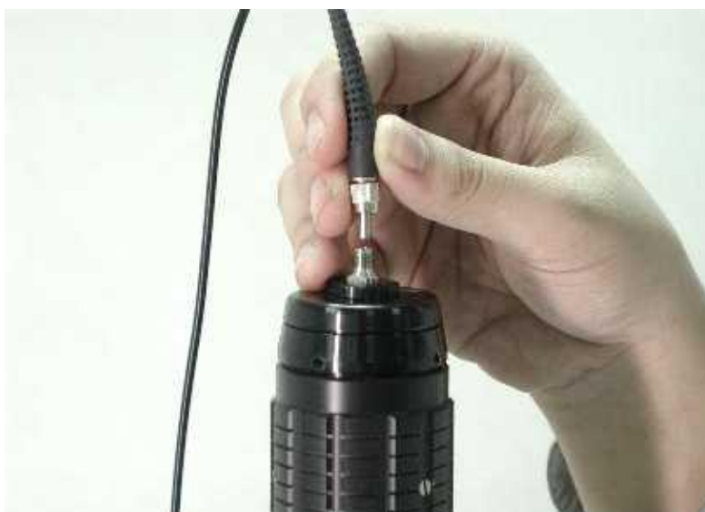
Figure 5.24 Attach the Delivery fiber to the Zoom unit
