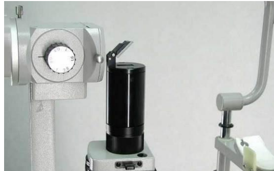
Figure 5.14 (b) New modified Illumination Tower fitted
