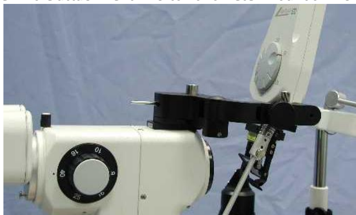
Figure 5.16 (c) Lightmed SYL9000 Mounting the whole attachment LDU to Tonometer mount & micromanipulator
