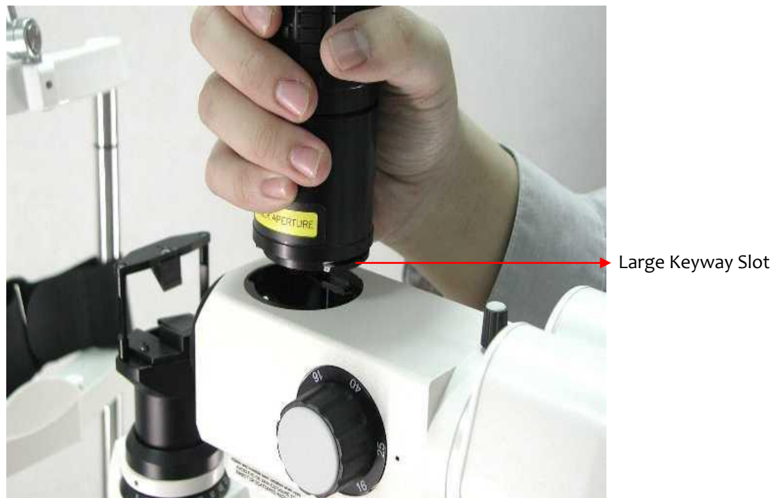
Figure 5.12 Align the keyways then fit the Zoom unit to the Delivery housing
