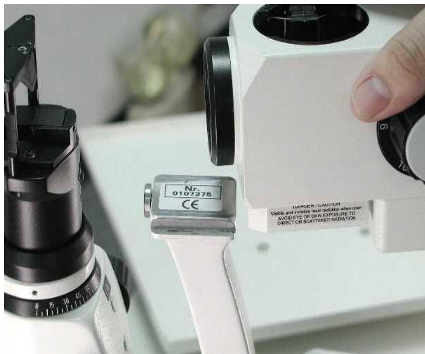
Figure 5.10 Fit Delivery unit housing to the Slitlamp
