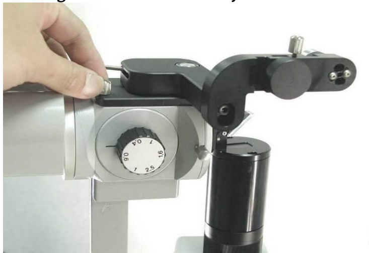
Figure 5.15 (b) Zeiss 30SL Attaching the Tonometer mount and Attachment LDU Mounting Arm
