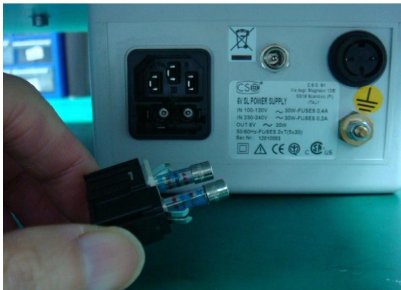
Figure 5.5 (b) Removal of fuse holder
