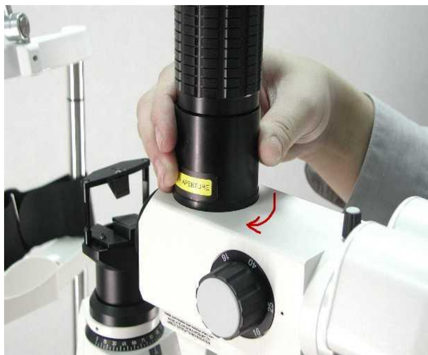
Figure 5.13 Rotate the Zoom housing to the end stop
