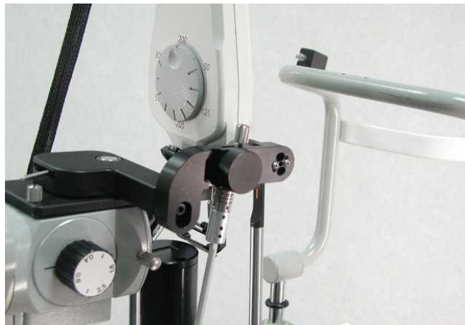
Figure 5.16 (b) Zeiss Style 30SL Mounting the whole attachment LDU to Tonometer mount & micromanipulator
