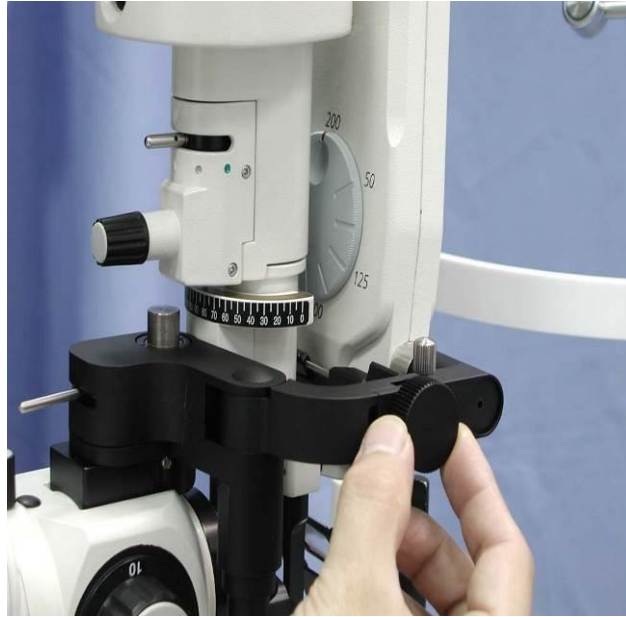
Figure 5.28(b) Old type Version Adjust the Attachment LDU Spot Size Focus using the knob on the mounting arm
