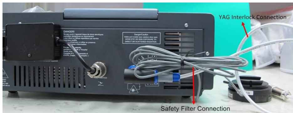
Figure 5.21 (b) Combo System Y-Joint connection set-up
