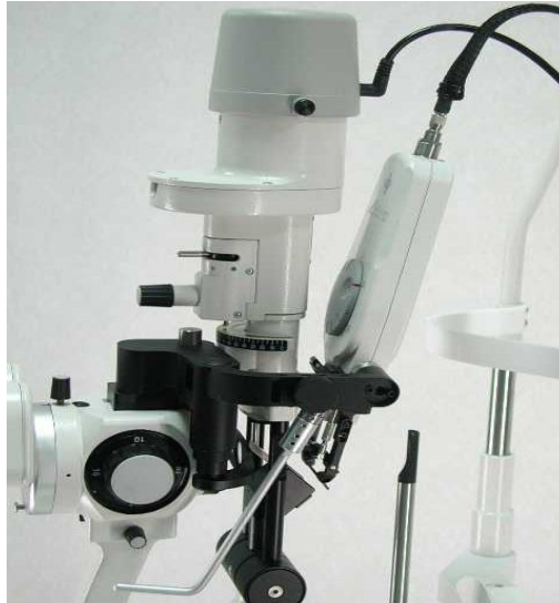
Figure 5.16 (a) Haag Streit Mounting the whole attachment LDU to Tonometer mount & micromanipulator
