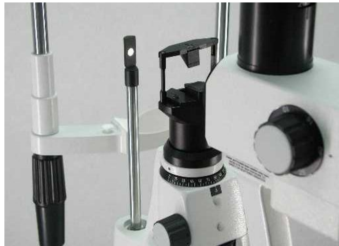
Figure 5.27 (a) Checking Field of View set-up
