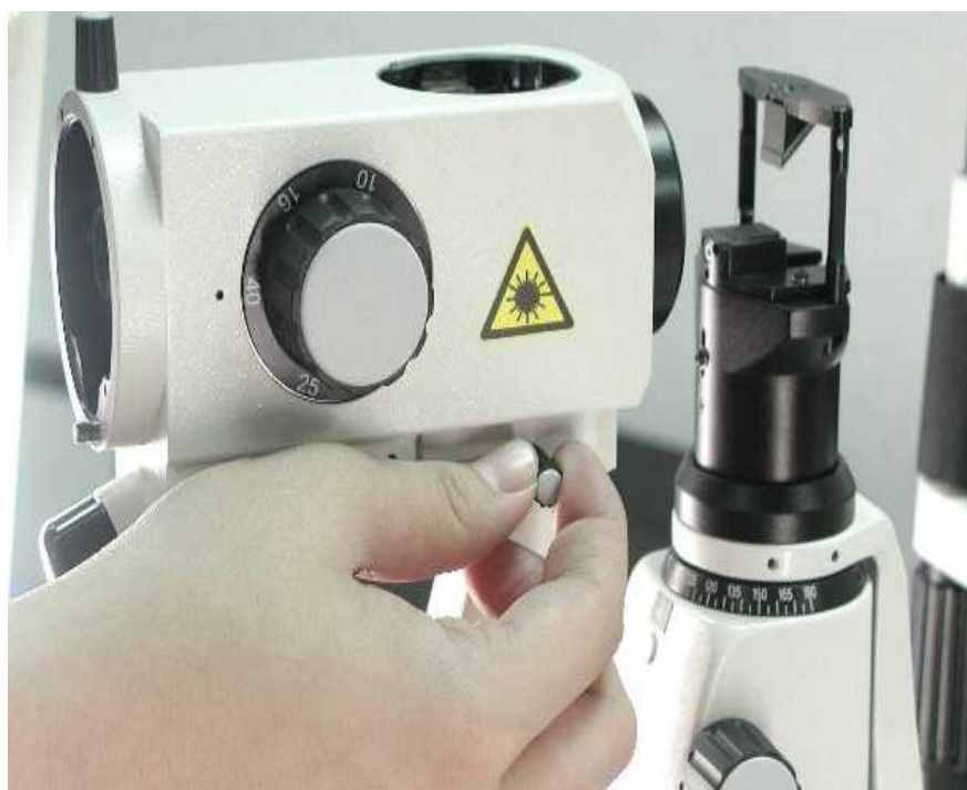
Figure 5.11 Lock the housing securely to the Slitlamp when it is pushed against Chrome Stop screw
