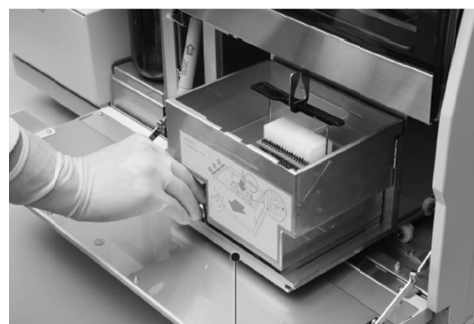
Loading station receiver
