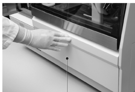
Loading station access door
