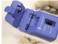
Inserting Fiber into Pull-Back Device
